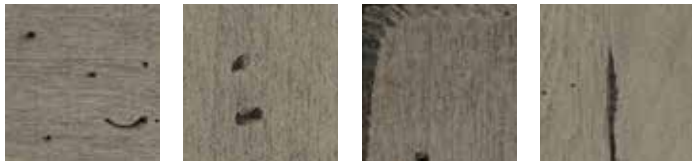
Wormholes Dents Rasping Mars & Splits Shown on stained finish
